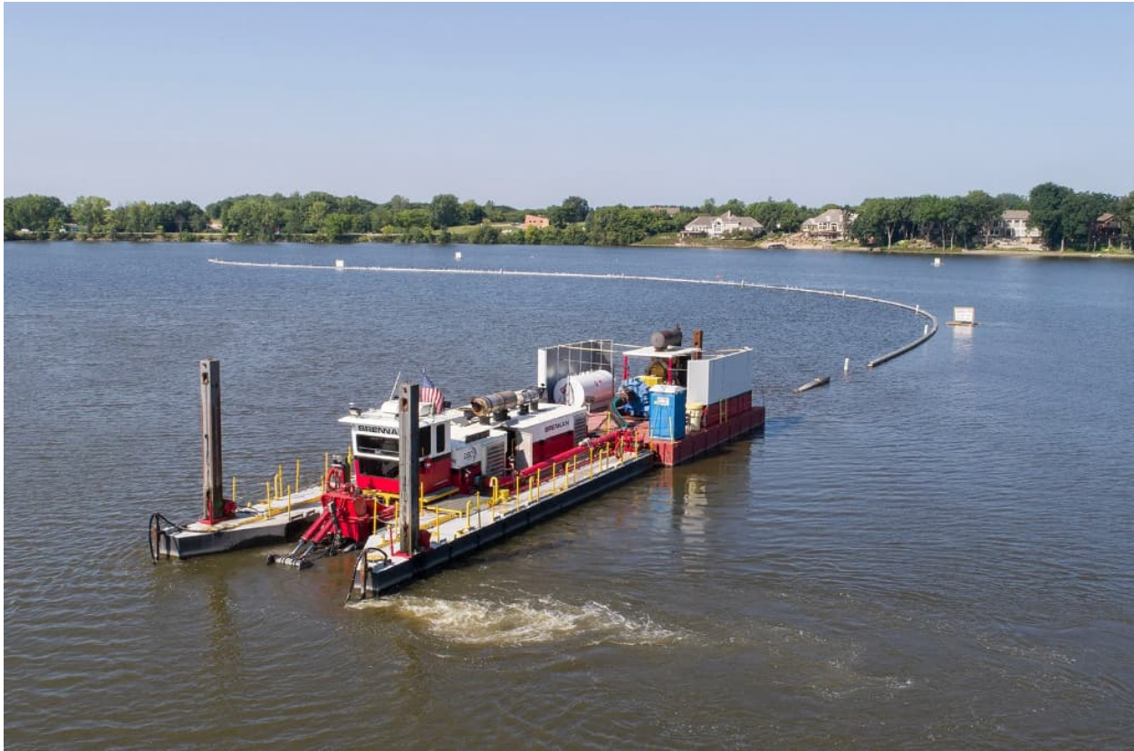
Figure 1: Example of a cutter head hydraulic dredge with floating HDPE pipeline
